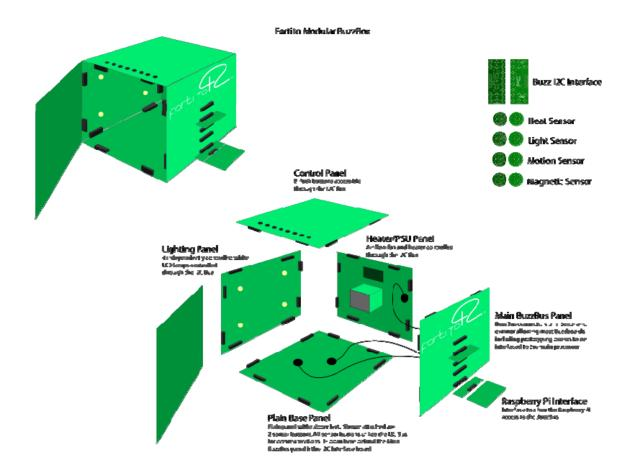
The *Buzz-Box* system is illustrated above. It consists of a set of identical 'plug-together' panels (25x25cm or 10x10 inches) that enable boxes of various sizes to be constructed. An innovative feature of these panels is that they are electronic circuit boards which can be customised with sensors, effectors and processors as desired (one common smart-home configuration is depicted).
