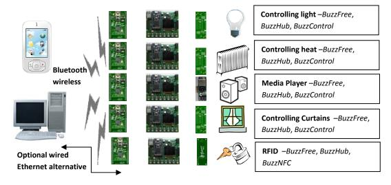
By using other *Buzz-Boards*, different smart-home functions can be controlled (eg there are a range of sensor options and other effectors such as *Buzz-IR* that enables appliances with infra-red remote controls to be managed). Thus using Buzz-Boards it's simple to construct a basic smart-home.
