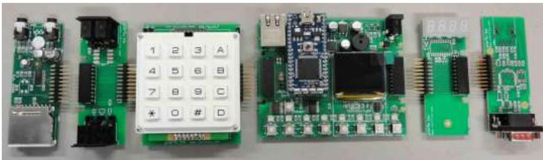
**Figure 1.** FortiTo Modules - From Left to Right Audio, Midi, Keypad, Base (Processor), LED & Network
