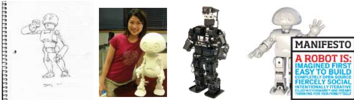
Figure 4: (from left to right) the original concept sketch, an early prototype (with Hsuan-Yi Wu), the production exoskeleton version (image courtesy of Trossen Robotics 9 )t and a version with a ‘Jimmy skin’ that mirrors the associated Maker book (image courtesy of Maker Media).
