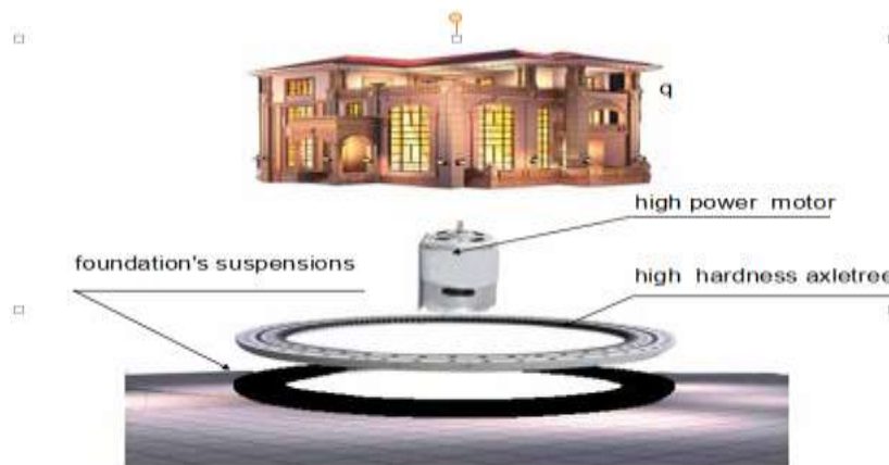
Figure 4. The foundation's suspensions and power system
