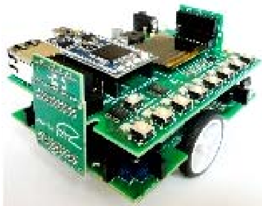
Figure 10. Mixed-reality Buzz-Board modules assembled as a mobile robot (Adapted from Callaghan 2012)
