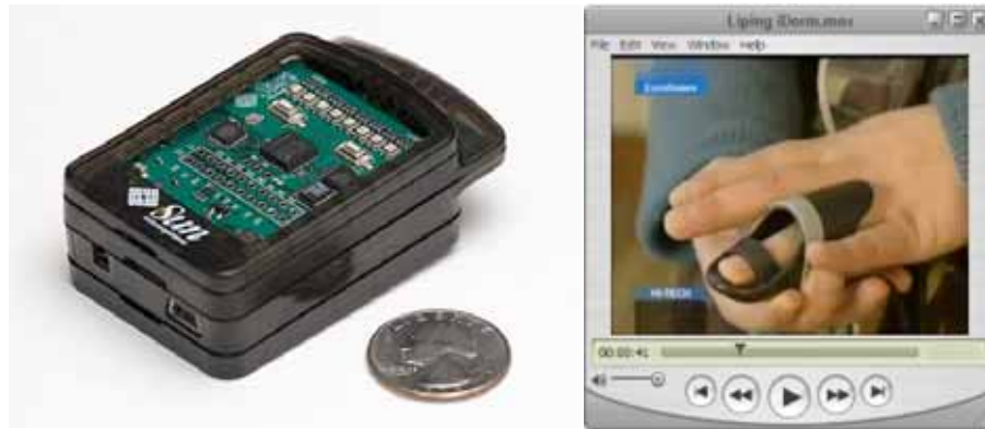
Figure 9 – The Physiological Emotion Sensing Hardware
