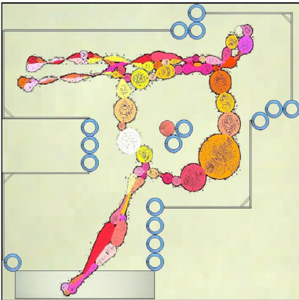
Figure 4: Perceptual map from an indoor test environment generated by the growing-cell-structure perception-space module and colour hue perception-signatures computed from the panoramic colour vision sensor.
