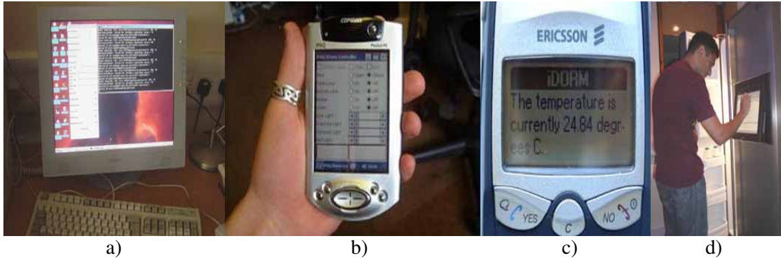
Fig. 3. a) PC based interface. b) Portable iPAQ interface. c) Mobile phone interface. d) iFridge interface.
