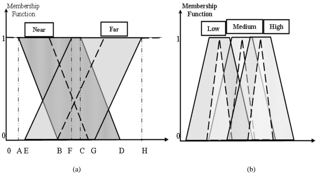
Figure (9): a) The input type-2 membership function for the input sensors for the edge following behaviours and the obstacle avoidance behaviour in indoor and outdoor robots. b) Output membership function for the velocities in the indoor robots.
