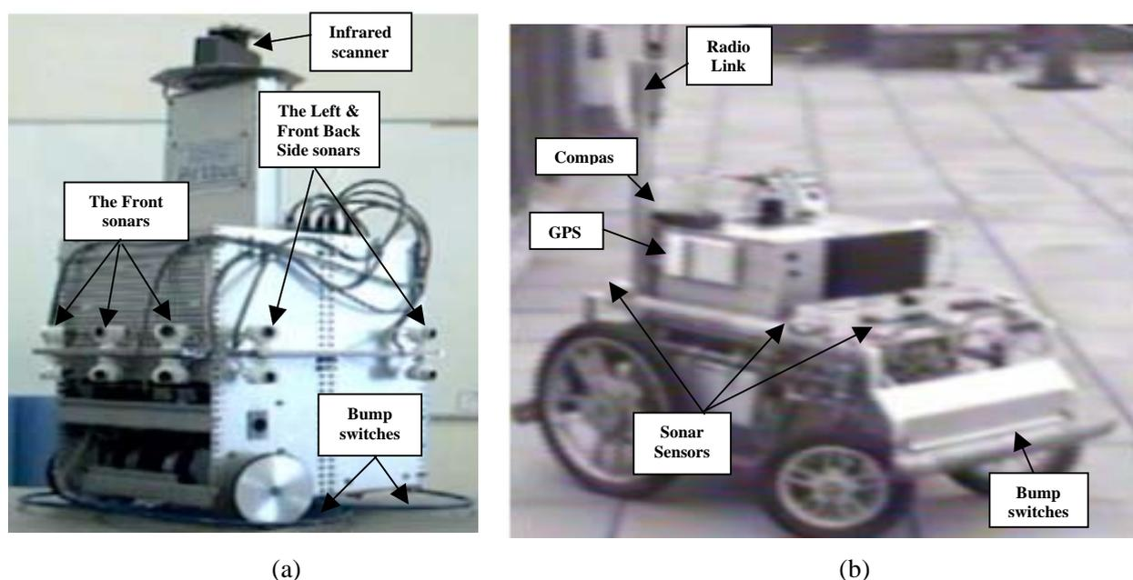
Figure (8): a) The indoor robot and its sensor configuration. b) The outdoor robot and its sensor configuration.
