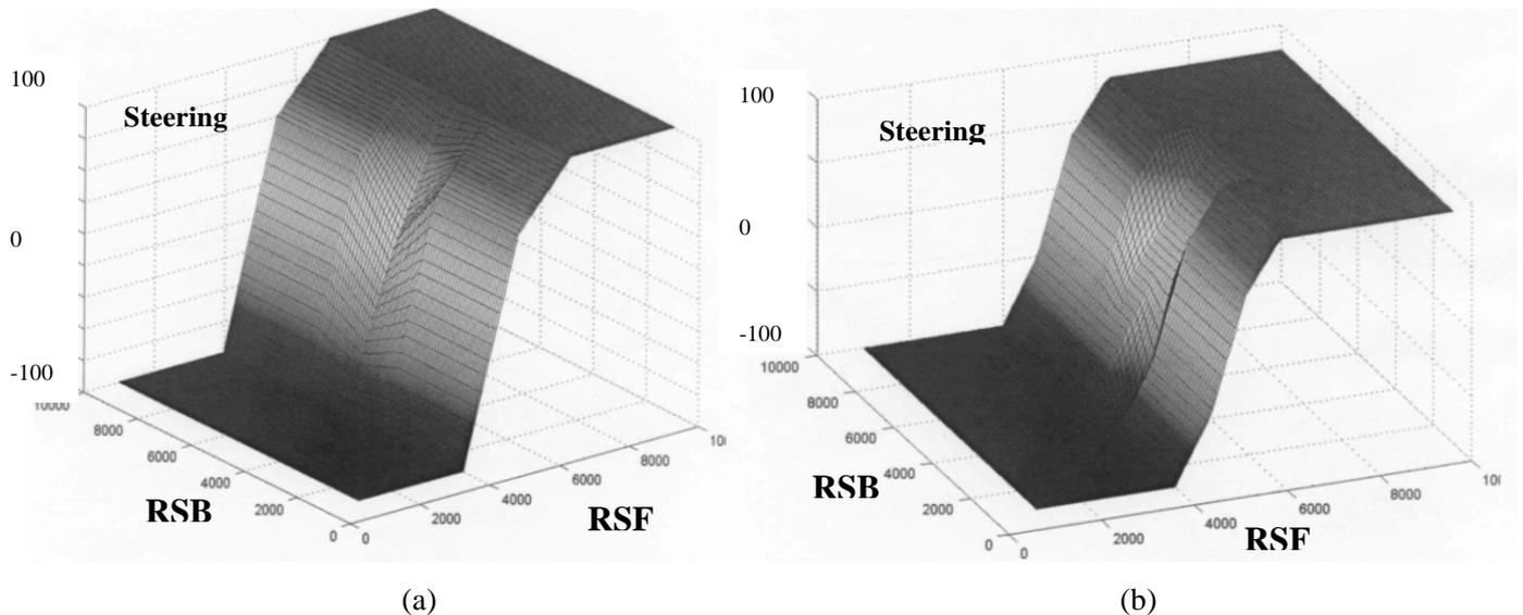
Figure (11): a) The Control Surface of a type-1 FLC using 3 fuzzy sets to represent each input.
