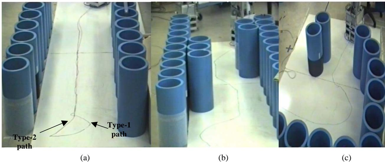
Figure (16): a) The indoor robot path using type-2 HFLC to follow a corridor and reaching a goal at the end the corridor. b) The path of the type-2 HFLC to follow a corridor while avoiding obstacles and reaching a goal at the end of the corridor. c) The path of the type-2 HFLC to follow an edge while avoiding obstacles and reaching a goal at the end of the edge.
