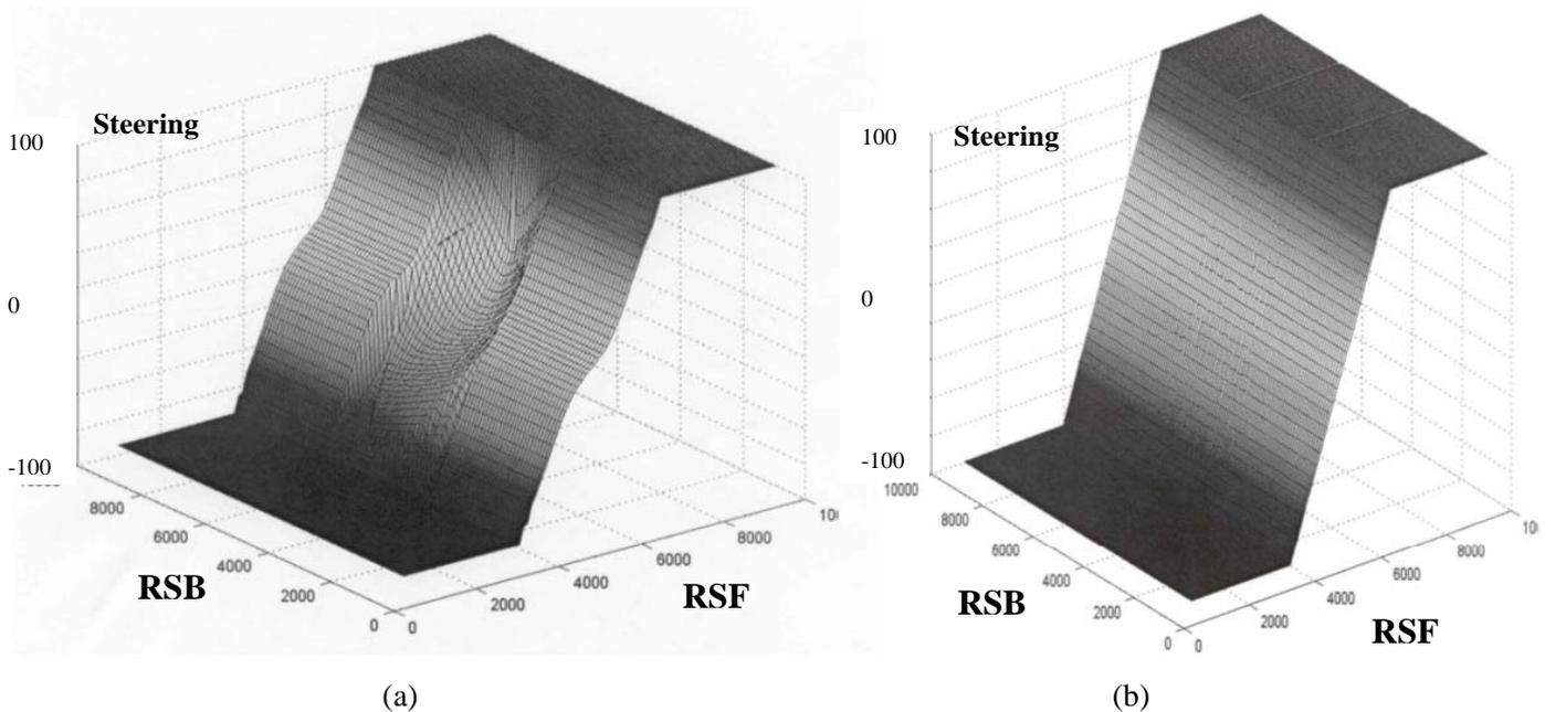
Figure (10): a) The Control Surface of a type-2 FLC for the right edge following behaviour. b) The Control Surface of a type-1 FLC using 2 fuzzy sets to represent each input.
