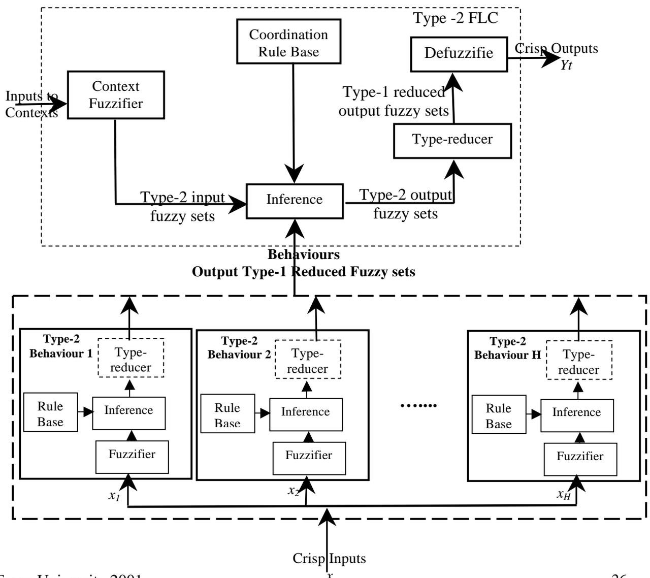
Figure (7): The type-2 Hierarchical Fuzzy Logic Controller architecture.
