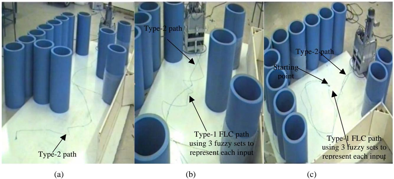
Figure (14): a) The indoor robot path using type-2 FLC to implement the obstacle avoidance behaviour.
