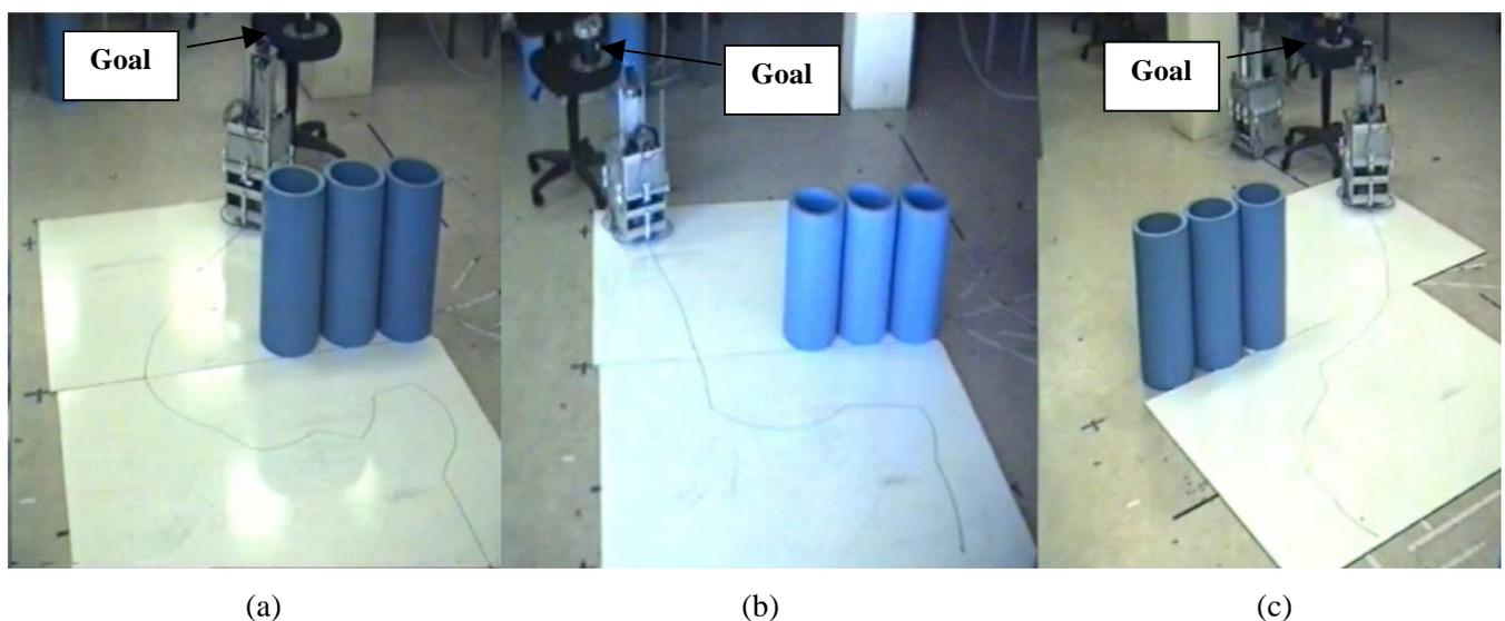
Figure (15):a) The indoor robot path using type-2 HFCL to reach a goal aligned with the robot. b) The robot path when the goal is to the left of the robot. c) The robot path when the goal is to the right of the robot.
