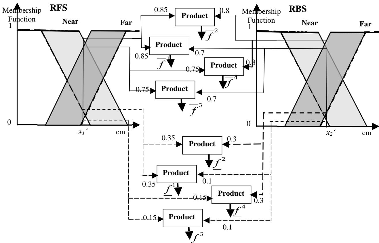
Figure(6): Pictorial description of fuzzification and inference operations for a robot type-2 FLC.
