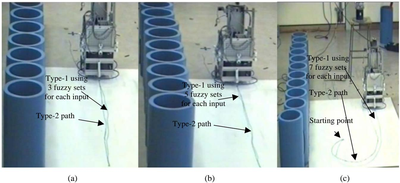
Figure (13): a) Indoor robot path using type-2 FLC to implement the left edge following behaviour compared against type-1 FLC path using 3 fuzzy sets to represent each input. b) The type-2 FLC path compared against type-1 FLC using 5 fuzzy sets to represent each input. c) The robot path using type-2 FLC to implement the goal seeking behaviours compared against a type-1 FLC using 7 fuzzy sets to represent the input.
