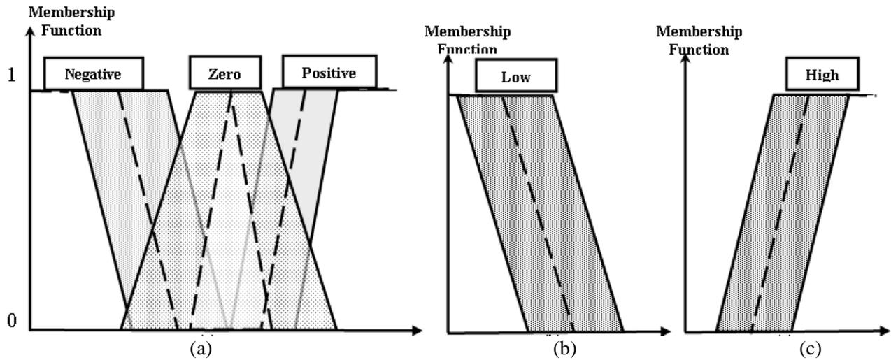
Figure (12): a) The type-2 input membership function for the goal seeking behaviour in the indoor and outdoor robots. b) The type-2 context fuzzy set for the obstacle avoidance behaviour and the right and left edge following behaviours. c) The type-2 context fuzzy set for the goal seeking behaviour.
