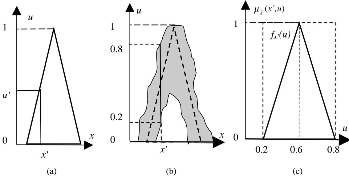
Figure (1): a) Type-1 membership function. b) Blurred type-1 membership function. c) Triangular secondary membership function plotted in thick line; interval secondary membership function plotted in dashed line
