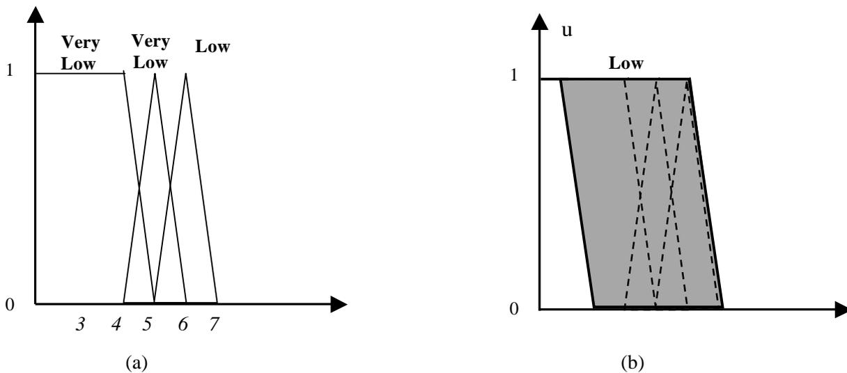
Figure(2): a) Three type-1 fuzzy sets representing an input to the FLC. b) The three type-1 fuzzy sets in Figure (2-a) are embedded in the LOW type-2 fuzzy set.
