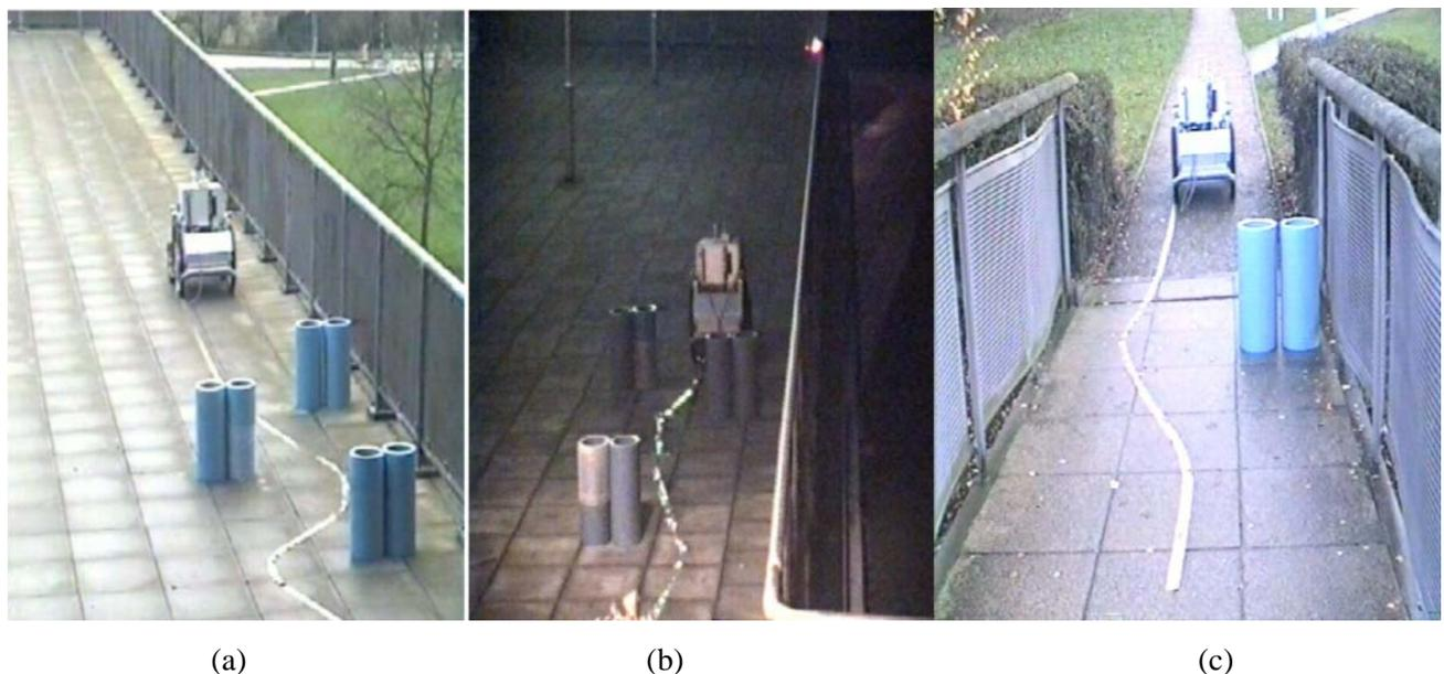
Figure (18): a) The outdoor robot path using the HFLC to follow an edge while avoiding obstacles. b) The same experiment as in Figure (18-a) carried during night using different obstacles configurations. c) The outdoor robot path using the HFLC to follow an irregular corridor while avoiding obstacles
