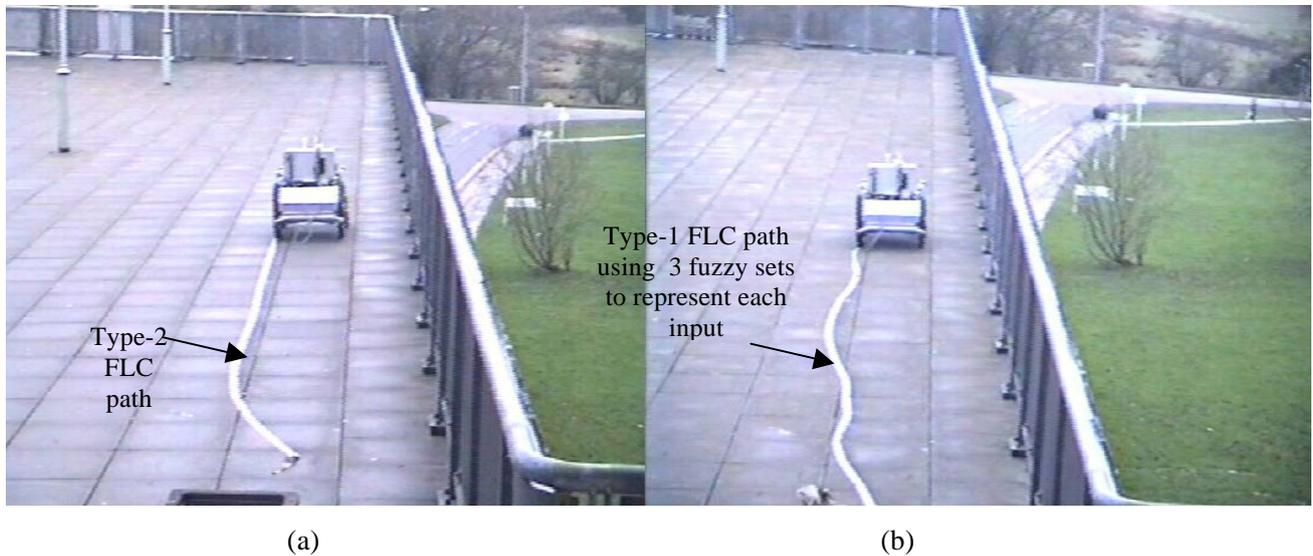
Figure (17): a) The outdoor robot path using type-2 FLC to implement the right edge following behaviour to follow an irregular edge. b) The robot path using a type-1 FLC which gave a bad response when the environment changed (windy weather).
