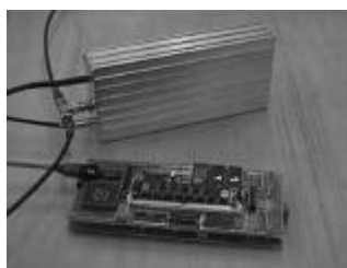
Figure 1 - University of Essex Prototype building services agent
