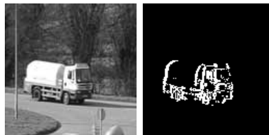
Fig. 1. Simple subtraction of point values for motion segmentation
