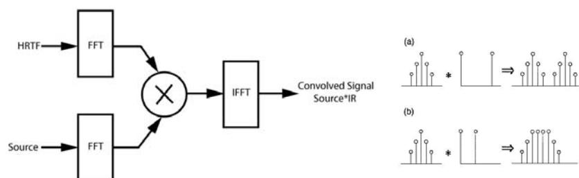
Figure 10. Convolution and output signal
