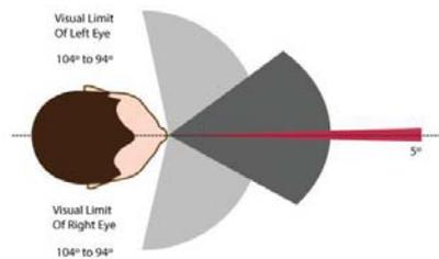
**Figure 1.** Horizontal Field of View.
