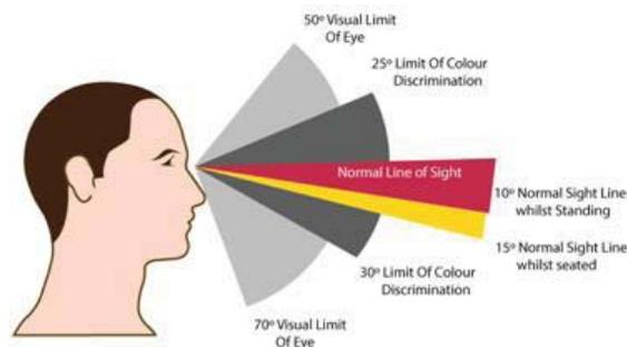
**Figure 3.** Vertical Field of View.
