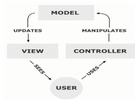
Figure 4 The Model-View-Controller Architecture
