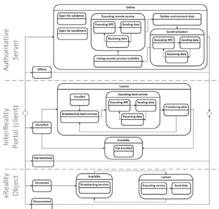
Figure 2. Blended Reality Distributed System states diagram
