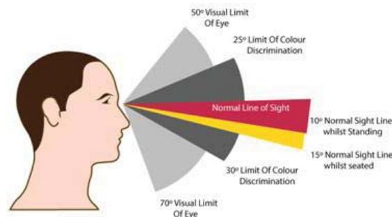
**Figure 3.** Vertical Field of View.
