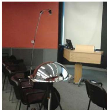
Figure 4. Spherical mirror and camera in room setup.
