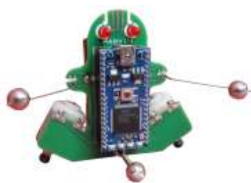
Figure 5 –A $35 robot constructed from FortiTo's BuzzBoard rapid prototyping kit
