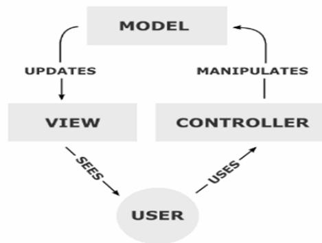
Figure 4 The Model-View-Controller Architecture
