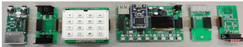
**Figure 2** Some BuzzBoard Internet-of-Things Components (an Internet Radio)
