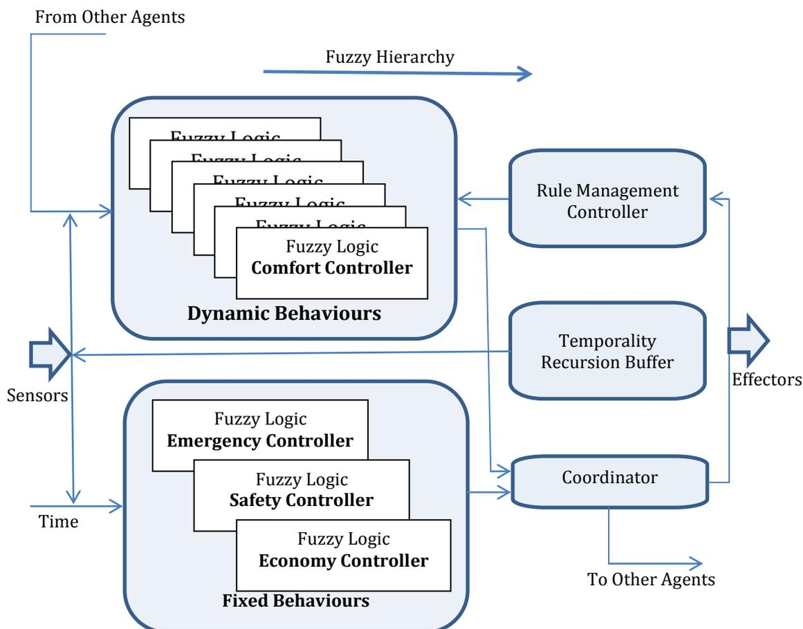
Figure 2: A Fuzzy Logic Implementation of a Behaviour Based Agent
