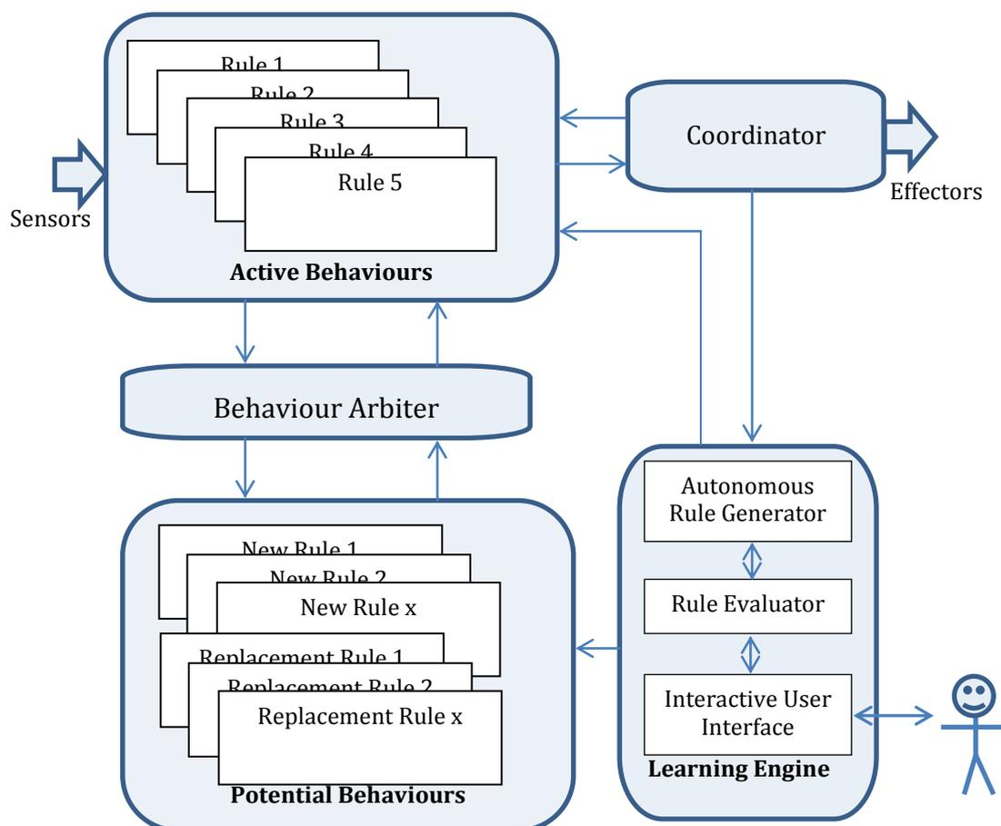
Figure 4 Adjustable-autonomy Behaviour-Based Agent
