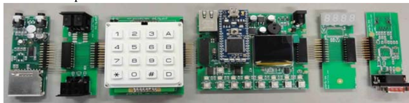
Figure 3 Some BuzzBoard Internet-of-Things Components (an Internet Radio)
