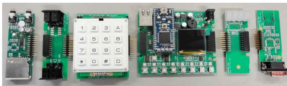
Figure 2. Buzz Board Examples (Audio, Midi, Keypad, Processor, LED & Network Boards)
