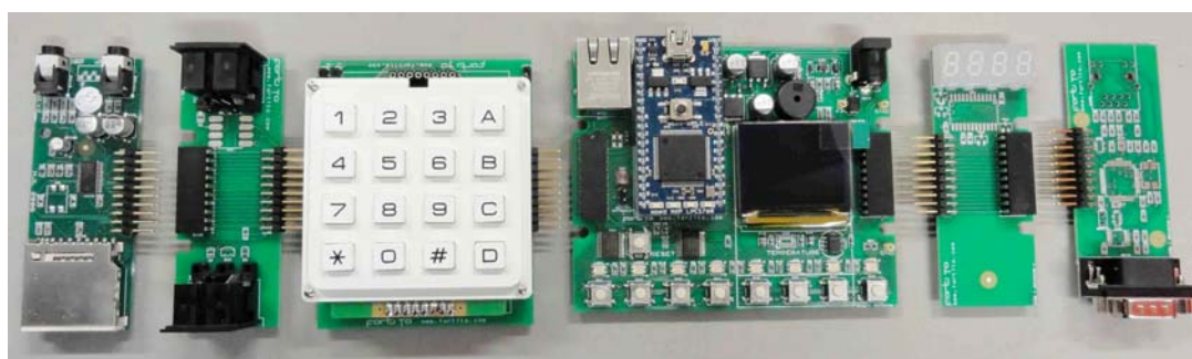
Figure 1. Buzz-Board Examples - From Left to Right Audio, Midi, Keypad, Base (Processor), LED & Network
