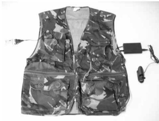
Figure 3. The XVEST. Physiological signals are acquired via the fingerclip and sent to a PC using the Bluetooth transmitter (left). Batteries are inside lower pockets.
