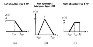
Fig. 4. (a) Type-1 left-shoulder MF. (b) Non symmetric triangular type-1 MF. (c) Right-shoulder type-1 MF [5].
