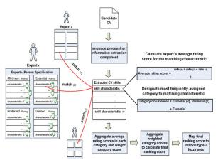
Fig. 6. Flow diagram showing the process for scoring and ranking CVs.
