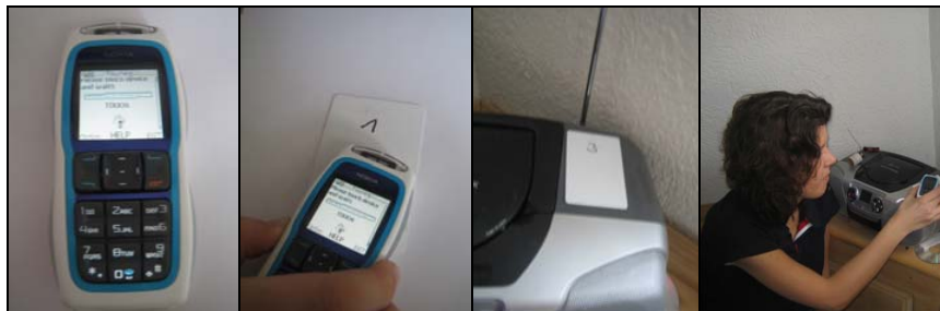
Fig. 7. The Nokia 3220 with integrated NFC chip, usage of the NFC phone for reading a Mifare NFC tag, a Mifare NFC tag attached to an smart object and a user who is using the NFC phone to touch the NFC tag.
