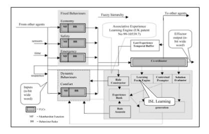
Figure 3 - An Embedded-Agent architecture for Intelligent-Artefacts
