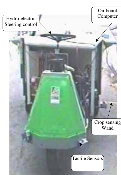
Figure (5): The outdoor diesel robot.
